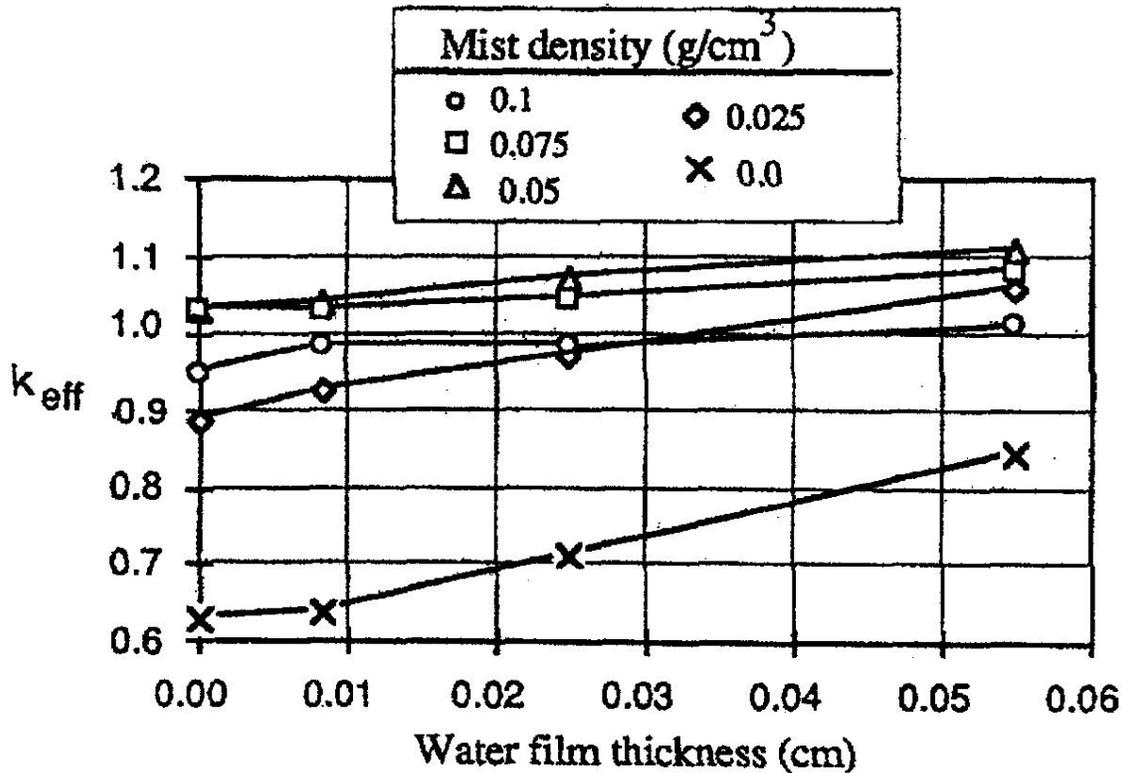
**Figure 3. Film Effects of Water Sprinklers on Storage Array of 4.1%-enriched UO<sub>2</sub> Rods**
