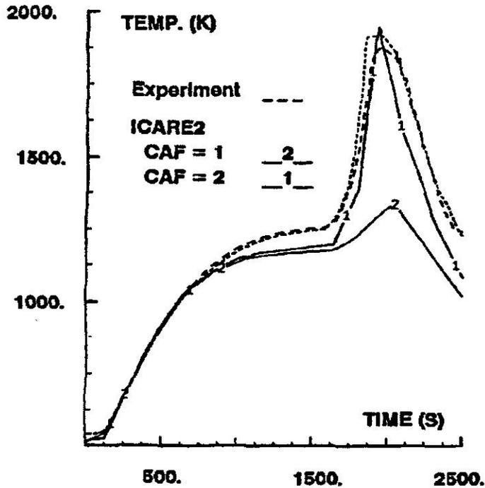
**Figure 5. Local Cladding Temperature vs. Time in the PHEBUS B9R-2 Test<sup>281</sup>**
