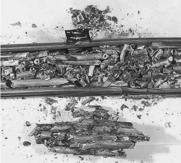
**Figure 4. Zirconium Fuel Rod Simulators that Incurred Runaway Oxidation**
