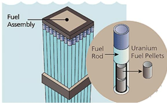
**Figure 1. Fuel Assembly, Fuel Rod, and Uranium Dioxide Fuel Pellets**<sup>75</sup>
