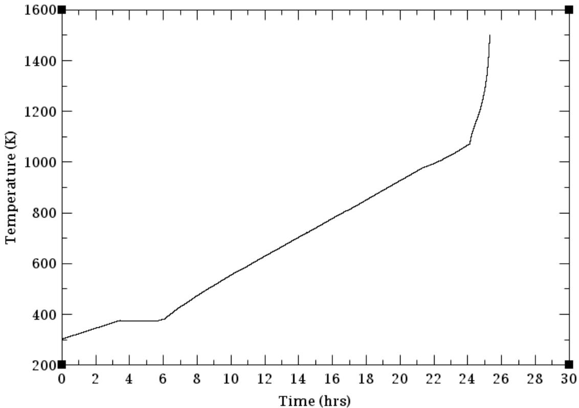
**Figure 2. Local Cladding Temperature vs. Time in the TRACE Simulation<sup>107</sup>**
